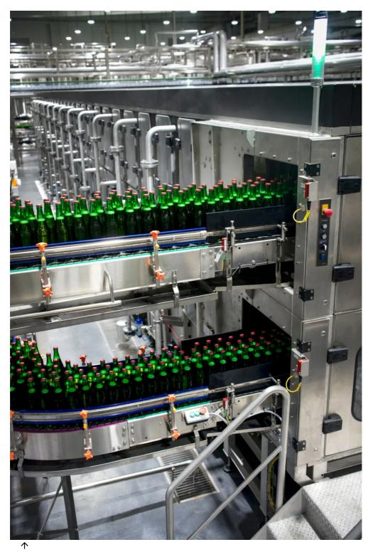
The returnable glass lines from KHS each feature an Innoclean DM bottle washer plus process technology, tunnel pasteurizers and cold glue labelers, among other machinery.
