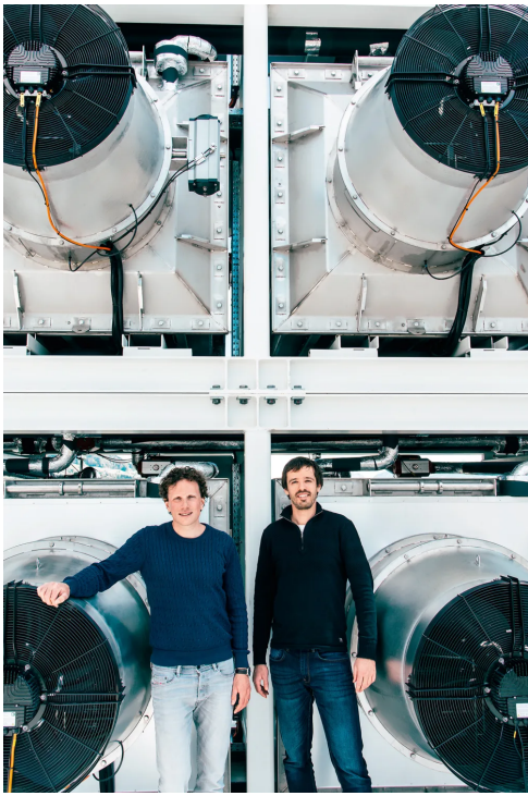
↑ Climeworks founders Christoph Gebald (left) and Jan Wurzbacher in front of their direct air capture filter modules in Hinwil, Switzerland.
