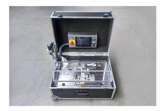
Turther development of the sequential overhaul of filling valves means a single kit can be used for different types of filling valve – a major benefit for production sites with several types of filler.
