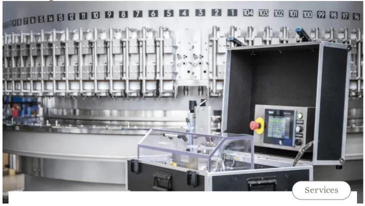
SEQUENTIAL OVERHAUL OF FILLING VALVES
