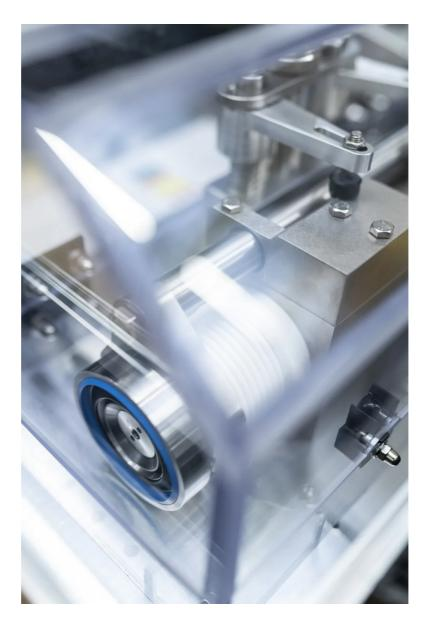
↑ Suitable for all valve types: a new adapter plate decouples the filling valve from the base plate of the test device.
