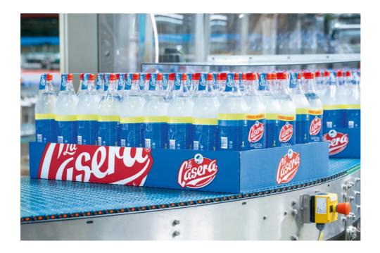
The DisplayPacker places big packs directly onto cardboard trays without these having to be further stabilized by a wrapping of shrink film.
