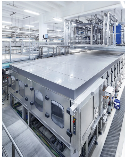
↑ The KHS Innopas SX tunnel pasteurizer at Mattoni 1873 ensures - optimum microbiological safety in the filled beverage cans.
