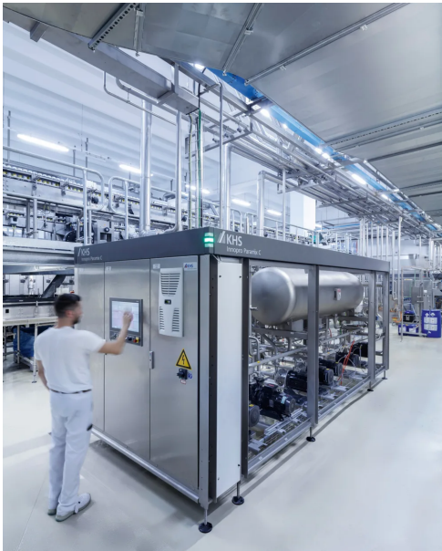
↑ Various ingredients are added to Mattoni 1873's soft drinks on the KHS Innopro Paramix C blending system.
