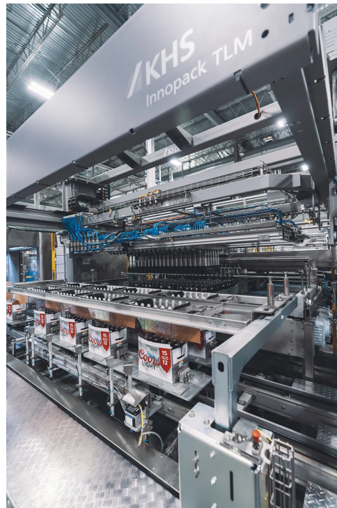
↑ The Innopack TLM is particularly flexible, a combination of a pick-and-place packer blocked with a Schubert erecting and closing module.
