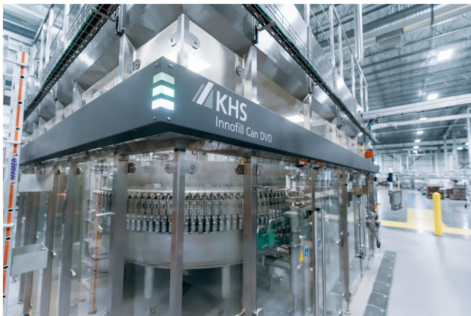
↑ The heart of the canning line is the KHS Innofill Can DVD filler that can process up to 72,000 cans per hour in many different sizes and formats.
