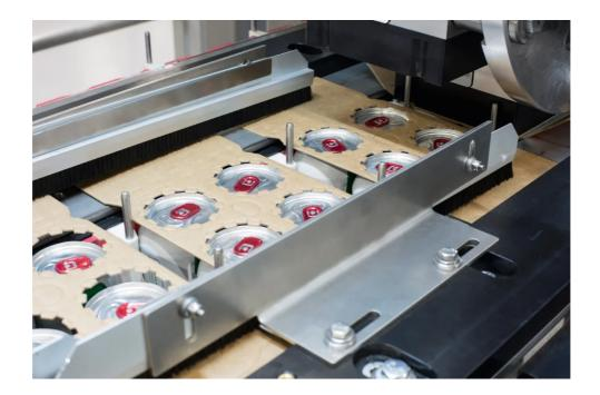
The cardboard clips or toppers are positioned on the cans before the wheel clamps their 'claws' under the rim of the can and erects the top.
