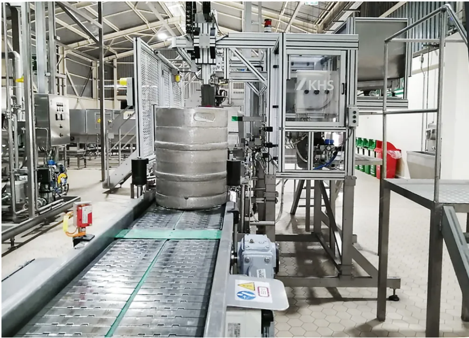
↑ The filled kegs are fed to the closure system on the KHS line.
