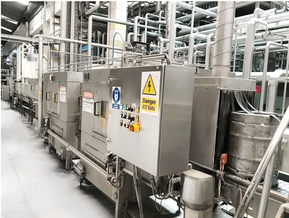
↑ Among the KHS equipment delivered to EABL is the Innokeg AK-3 exterior keg washer for the high-capacity range, here on the line installed in 2005.
