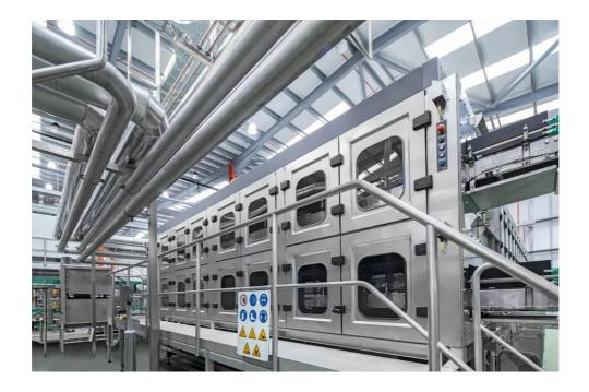
The extremely flexible Innopas SX pasteurizer permits very fast product changeovers and can be expanded at a later datethanks to its modular design.
