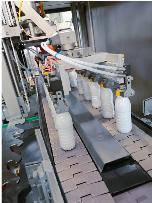
↑ Filled and capped PET bottles leaving the stretch blow molder/filler block on their way to the sleever.
