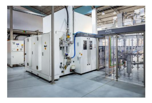
↑ The InnoPET BloFill PET block from KHS permits up to 36,000 bottles to be manufactured and filled per hour.
