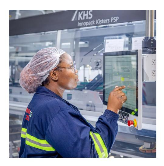
↑ With its role-based access system, the ClearLine HMI (Human Machine Interface) facilitates the operation of KHS systems such as the Innopack PSP Advanced shrink packer.
