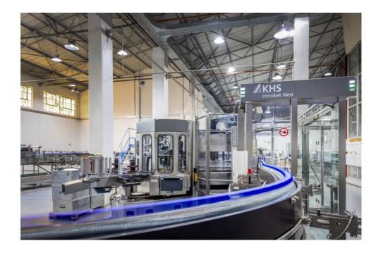
The Innoket Neo labeler with a rollfed station ensures precise and efficient hot-melt, wrap-around labeling of PET bottles.
