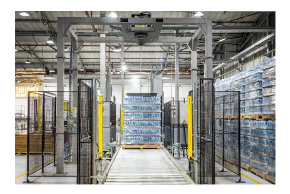
Special PET bottles call for nonstandard shapes and sizes of pallet which the palletizer was perfectly adapted to using individual robot programming.
