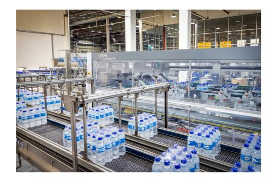
The Proven efficiency: the modular Innopack PSP Advanced packaging machine processes up to 14,400 packs per hour.
