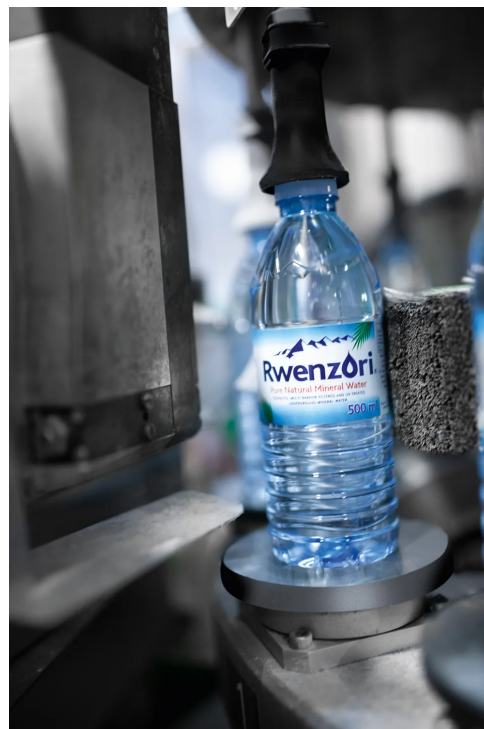
↑ Paper labels are glued and brushed onto Rwenzori's bottles on a KHS Innoket Neo labeler.
