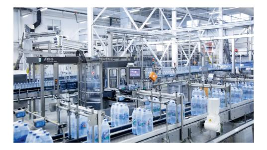
↑ Non-stop production thanks to the KHS labeler with its double station and automatic changeovers.
