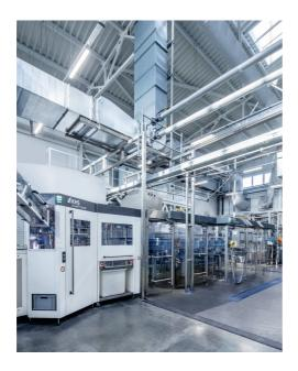
↑ Minimizes product loss: the InnoPET BloFill stretch blow molder/filler block from KHS.
