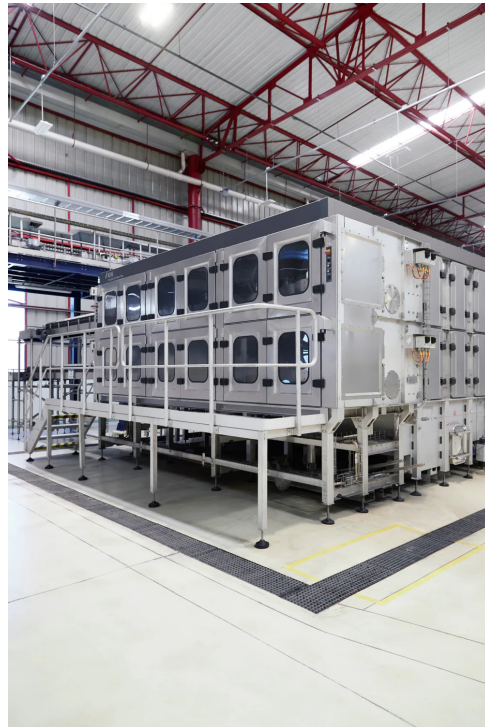
↑ The KHS Innopas SX tunnel pasteurizer at CCU ensures optimum microbiological safety in the filled beer cans.
