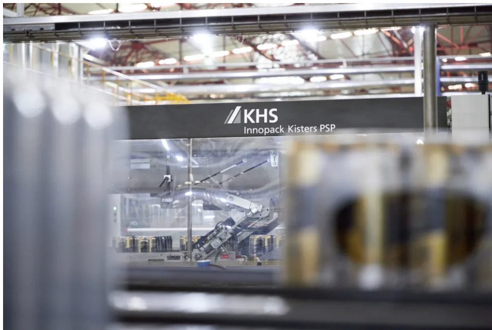
↑ On the KHS Innopack Kisters PSP packer the cans are placed on pads and wrapped in film.
