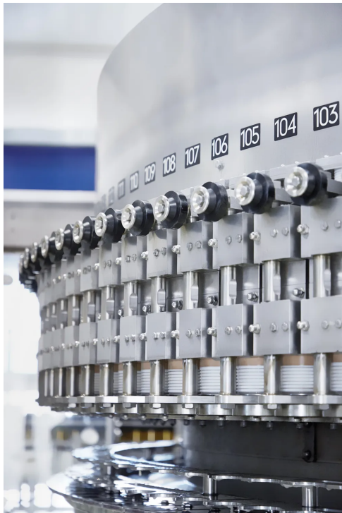
↑ The KHS Innofill Can DVD filler processes up to 82,000 cans per hour.
