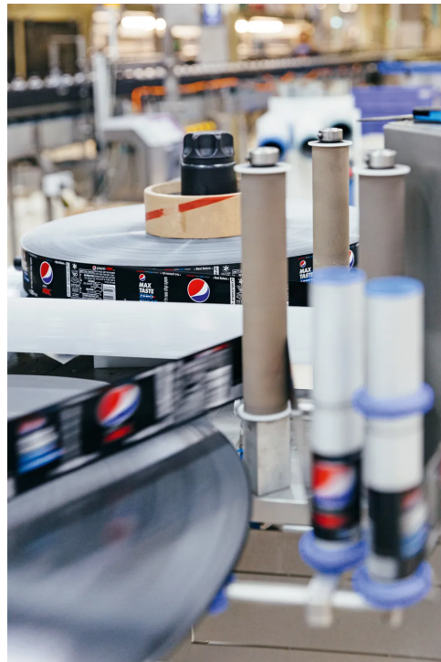
↑ On the Innoket Neo roll-fed labeling machine from KHS PET bottles filled with sugar-free Pepsi Max are dressed with their characteristic black labels.
