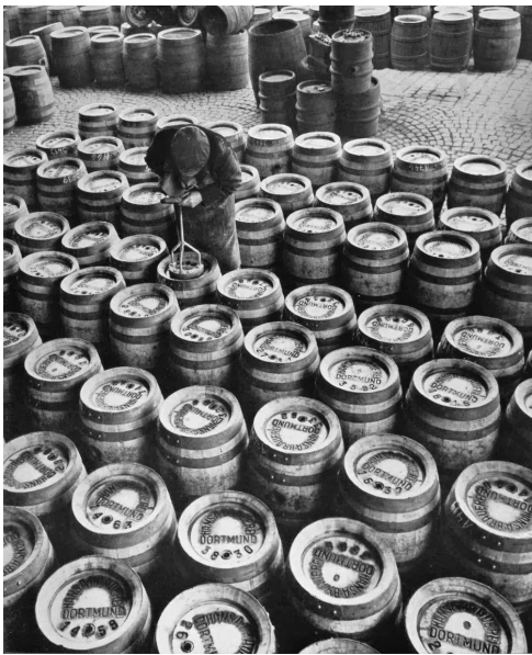
↑ At the Hansa Brewery new wooden barrels are branded with the company “brand” name by hand with the help of a branding iron.
