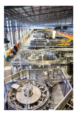
↑ The two KHS Innofill Glass DPG ECO fillers at the new production site in Marracuene form the hub of the impressive new line.
