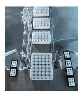
↑ With the help of four short conveyor belts, each with a separate electronic control, the packs are brought into position for access by the robot.
