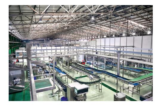
View of the line's packaging section: in the center is the labeler, with the packer to the right and the conveyors with buffer segments in front of and between the two.
