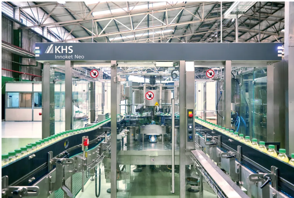
↑ The KHS Innoket Neo roll-fed labeler dresses the PET bottles on the line with labels.
