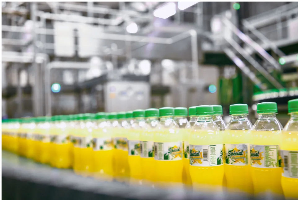
↑ On UCB's PET line water and soda pop are filled into four different sizes of bottle – here the 330-milliliter variant.
