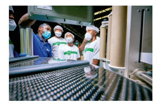
↑ A KHS service employee shows UCB operators how to change reels on the Innoket Neo for roll-fed labeling.
