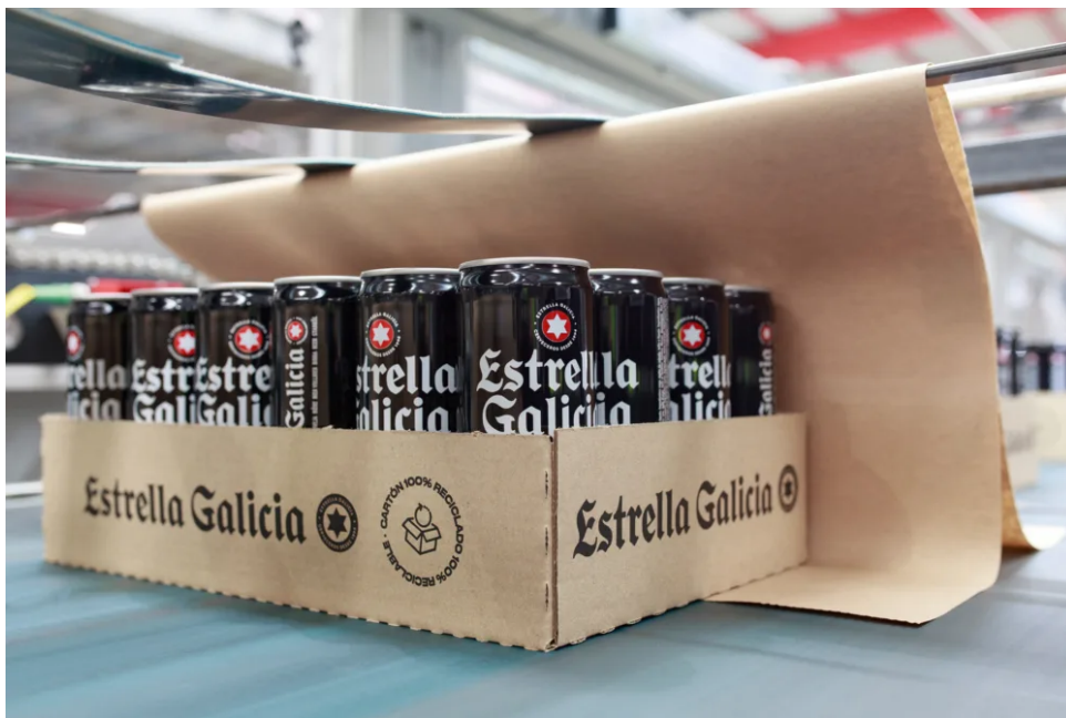
↑ The Innopack Kisters TSPP paper wrapping module wraps beverage cans in perfectly folded and glued paper instead of plastic film.
